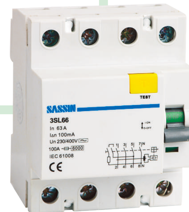
Residual current circuit breaker current rating: 100 A Inbuilt ON/OFF indication Inbuilt earth leakage Indication
